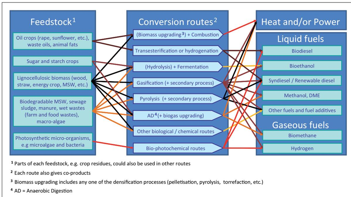
**Figure 3:** Schematic view of the wide variety of bioenergy routes. Source: E4tech, 2009.
