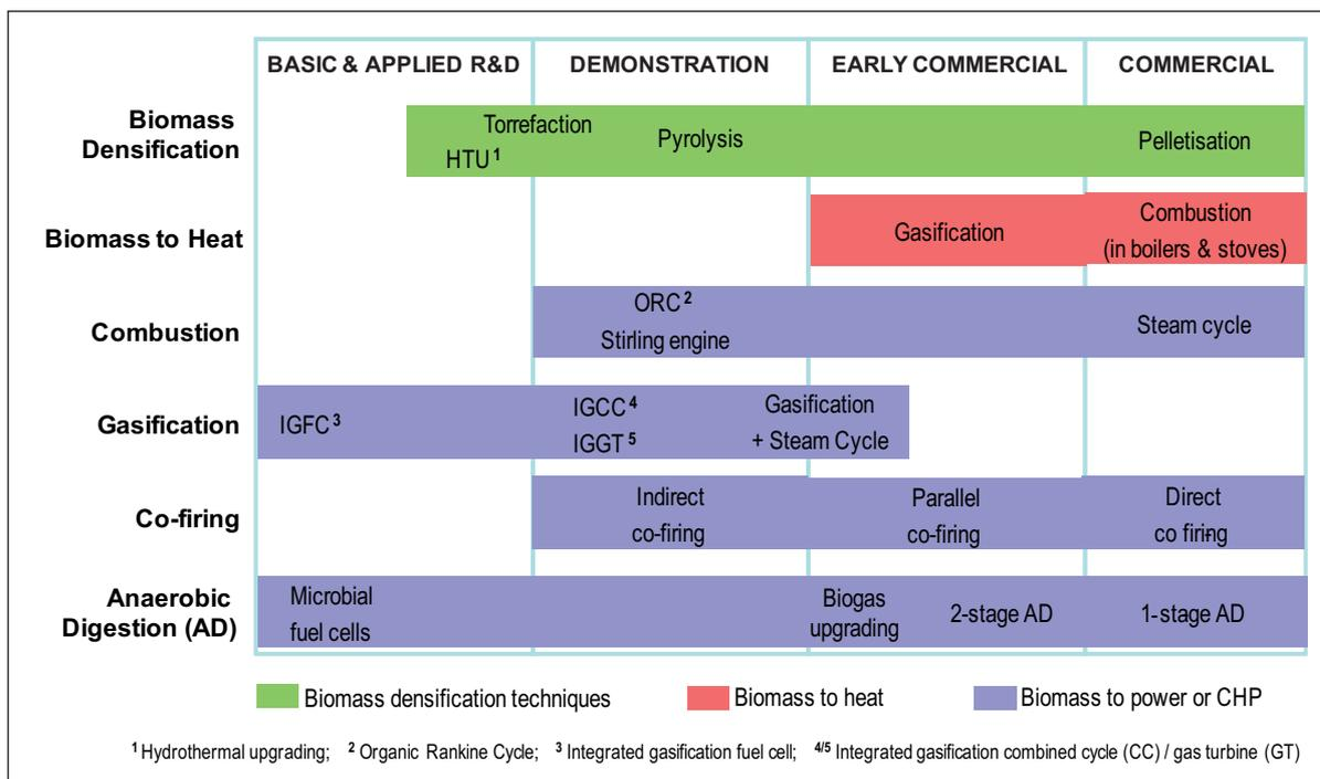
**Figure 4.** Development status of the main technologies to upgrade biomass and/or to convert it into heat and/or power. Source: E4tech, 2009.
